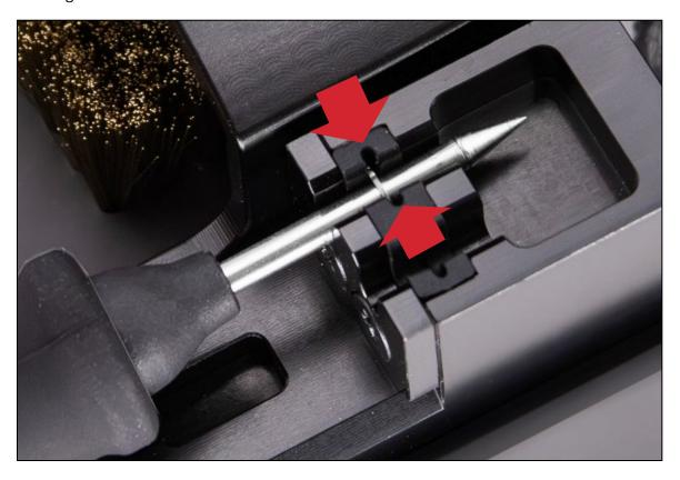
Carefully pull the handpiece backward, leaving the cartridge safely in the removal tool. You may need to steady the workstand with your other hand as you pull.
